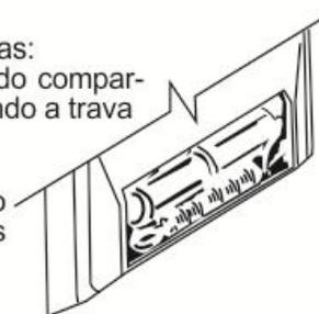
No modo pilha, verifique a posição correta da chave conforme indicado. Ch6 =
